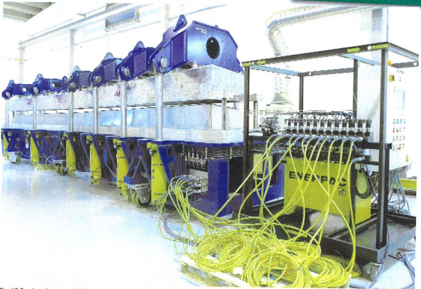
The 10.5 m long invar mould for Airbus composite manufacturing
